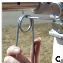
\*Pin should clip below casting
